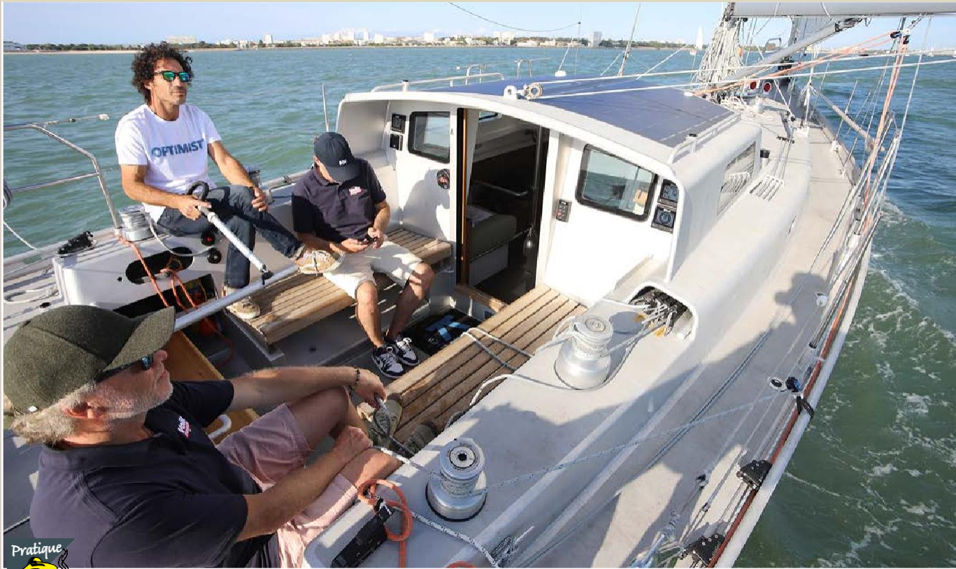
The cockpit is deep and well protected from the sea. The helm position on the gunwale is very high, providing a good view over the doghouse. Note the attention to detail, like the brushed finish of the winches, which are fitted to the aluminium coaming.
