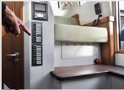
The electrical panel, installed halfway down the companionway, is exposed. It will be protected by a wooden washboard.
