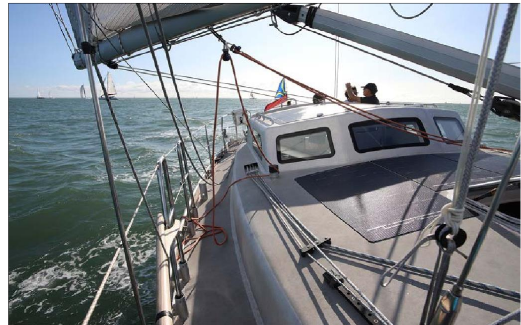
▲ On deck, we appreciate the finish of the aluminium, the surface of which has been sandblasted to eliminate the need for a non-slip coating. Note also the preventer guy, which is very reassuring when gybing.
