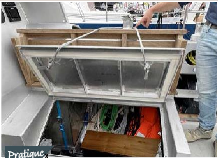
A simple way to secure the opening of the cockpit locker: a cable around the winch
